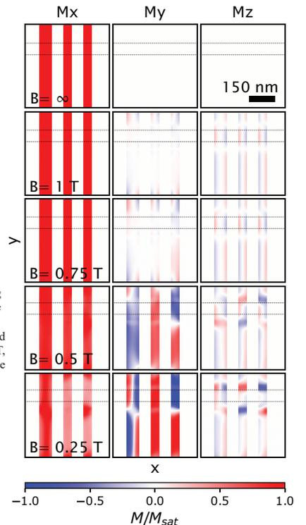
Figure 8: Simulated magnetization of cobalt gates normalized by the saturation magnetization.
