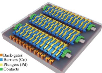
Figure 1: Proposed qubit array architecture based on Ultra-thin body SOI nanowires with magnetic gates.
