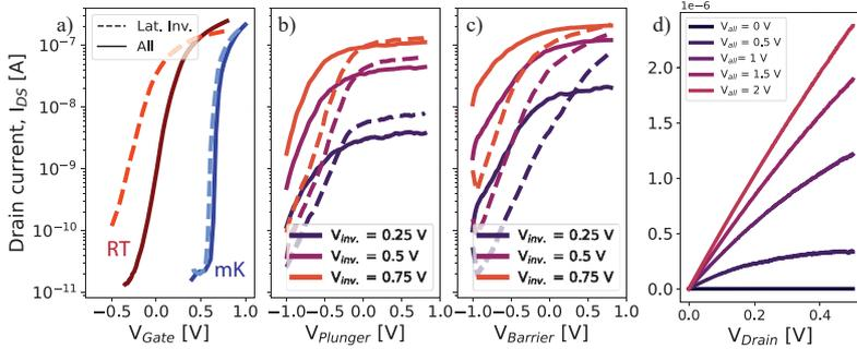
Figure 3: Pd and Co gates control at room temperature. a)  $I_{DS}-V_G$  for all gates and lateral inversion gates only. b, c)  $I_{DS}-V_G$  for plunger and barrier gates.  $V_{inv}$  denotes the voltage applied to all gates not included in the linear sweep, solid lines are for left gates, dotted lines for right gates. d)  $I_{DS}-V_{DS}$  for different bias applied to all gates.
