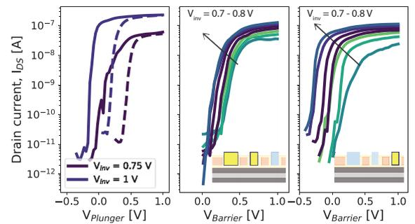
Figure 4: Gates control at mK showing the  $V_{th}$  dependence of barriers on plunger polarization.  $V_{inv}$  denotes the bias applied to all gates not included in the linear sweep.
