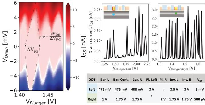
Figure 5: Basic Coulomb spectroscopy at 10 mK for the left and right dot (with grounded Source). The biases applied to gates for the dots formation are listed in the table.
