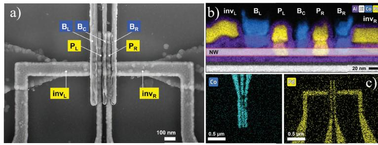
Figure 2: a) SEM image of the fabricated device. The left Co gate (60 nm wide) is 20 nm wider than the right one for the tuning of qubits' addressability. b) TEM cross section of the device with EDX analysis. The thickness of the nanowire and the BOX are 18 nm and 20 nm for an optimal electrostatic control. c) EDX-SEM analysis of the gated structure.
