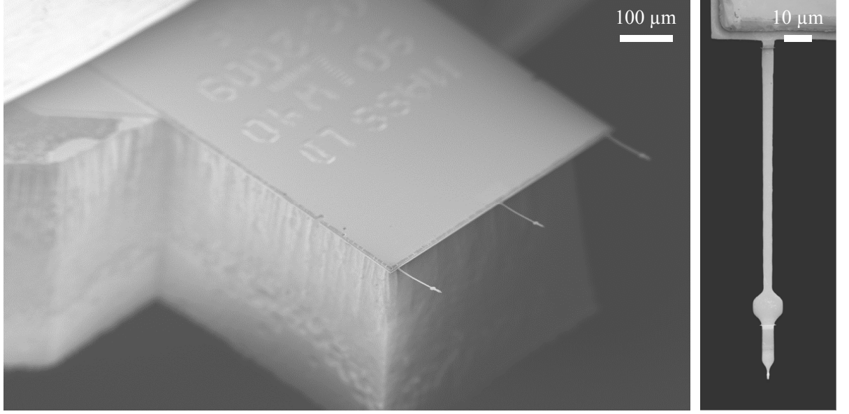
Figure 4.1. | SEM images of ultrasoft Si cantilevers held by a Si chip. On the right, detail of one cantilever.
