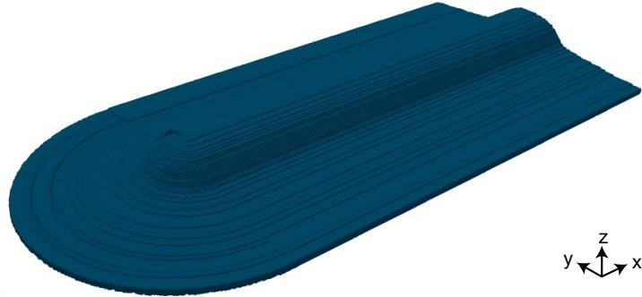
**FIGURE 5.12— Simulation of cobalt nanowire geometry including a thin sheet of “halo” in finite difference solver MuMax3.**
