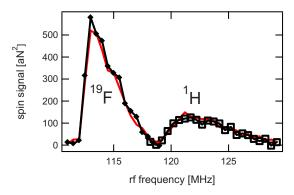
FIG. 4. (Color online) Simultaneous frequency scans of two nuclear species. With each solid diamond data point, exciting  $^{19}\mathrm{F}$  spins, an additional open square data point was measured, exciting  $^{1}\mathrm{H}$  spins. Points represent 20 min measurements taken simultaneously with two rf frequencies spaced by 7.2 MHz. The thin line represents data taken by scanning with a single rf frequency excitation. FM modulation was  $\Delta \nu = 1500 \, \mathrm{kHz}$ .
