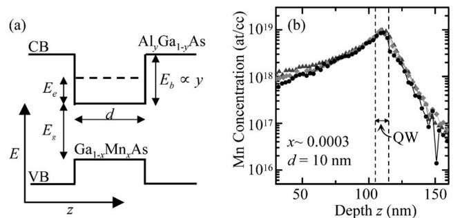
FIG. 1. (a) Schematic of the QW band structure, showing the well width  $d$ , the GaAs band gap  $E_g$ , the QW barrier height  $E_b$ , and the electron kinetic energy  $E_e$ . (b) SIMS Mn profiles for three  $d=10$  nm QWs for nominally the same Mn concentration  $x \sim 0.0003$ , with  $y=0.1$  (light gray),  $0.2$  (gray), and  $0.4$  (black).
