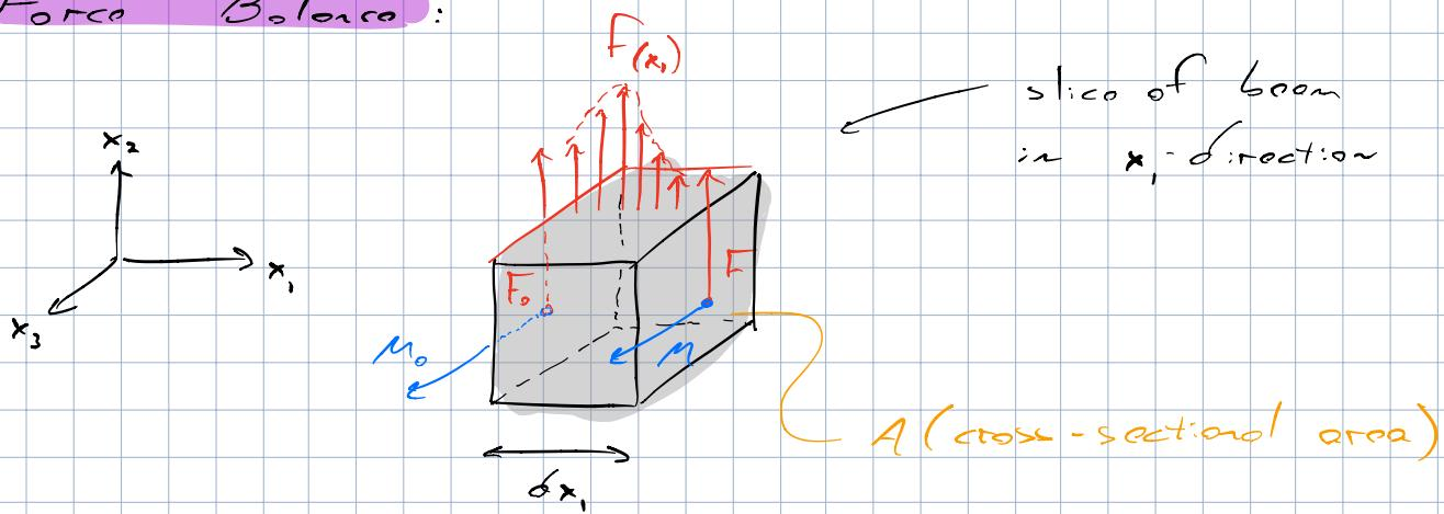
$$F_0 + \int_0^l f(x'_1) A dx'_1 - F(l) = 0 \quad \leftarrow \text{full beam}$$
