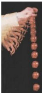
A falling apple captured by strobe photography at 60 flashes per second. The acceleration of the apple is indicated by the widening of the spaces between the images. (Estate of Harold E. Edgerton/Palm Press.)
