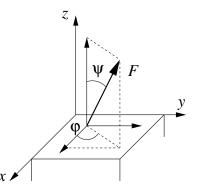
(a) Calculate the normal stress in z-direction and the shear stress in xand y-direction.
