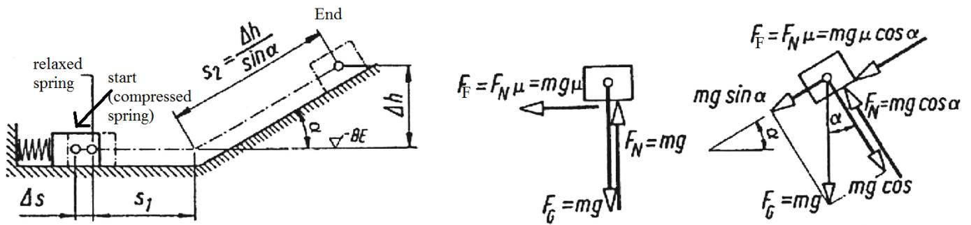
b) The energy at the end of the movement  $E_E$  is equal to the kinetic energy  $E_A$ , at the beginning, minus the loss due to the friction:
