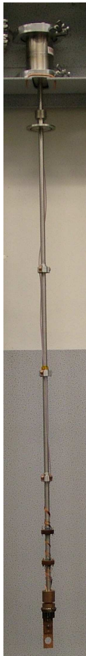
Figure C.12: An RF probe for Spectromag (model F2001).
