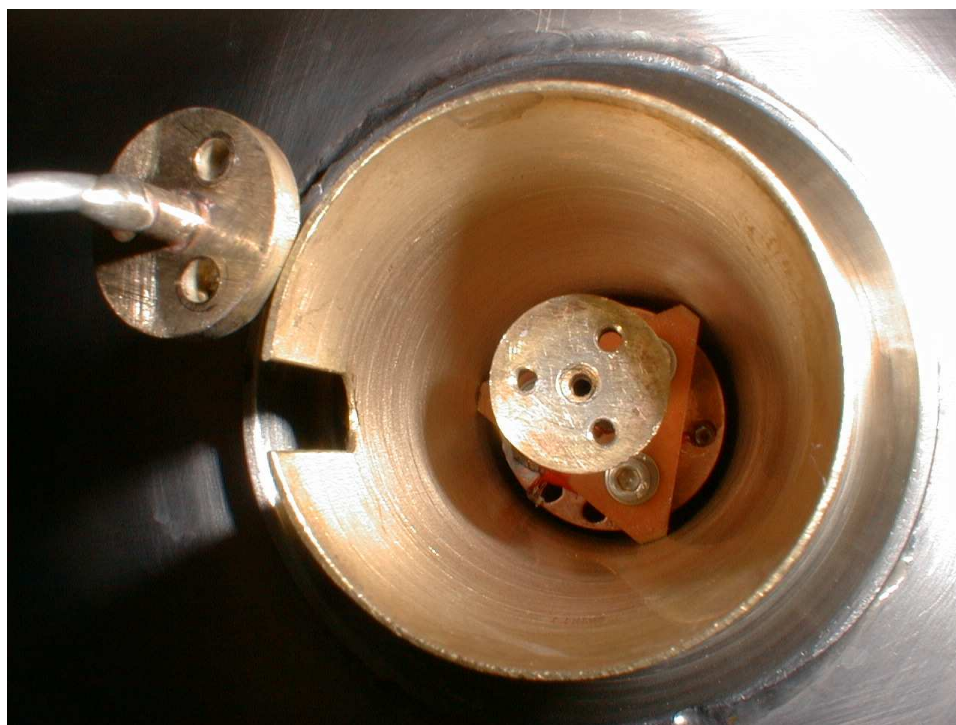
Figure C.2: A view from below the Spectromag of the two flanges involved in the indium seal. The flange in the center leads to the bottom of the VTI, while the flange on the left leads to a capillary attached to the NV assembly. Indium residue is visible on the center flange.
