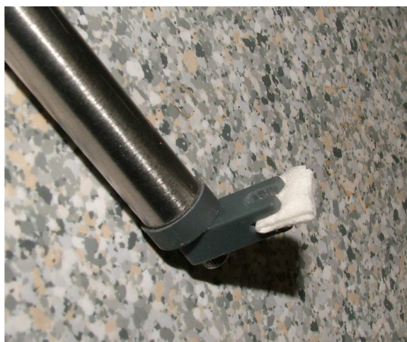
Figure C.9: The bottom of a VTI window cleaner with lens paper in place.
